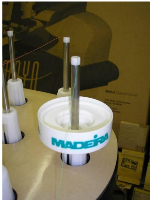
Pic. 2: Attaching the Madeira Spool/Cone Holder to the AMAYA
