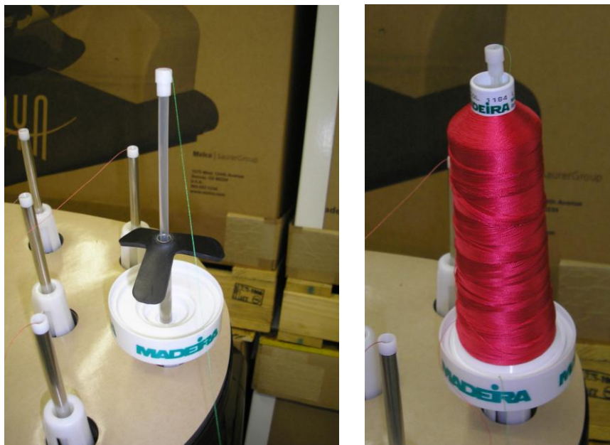
Pic. 10: Combination of Spool/Cone Holder with Thread Tree Clovers for older type Madeira thread cones
